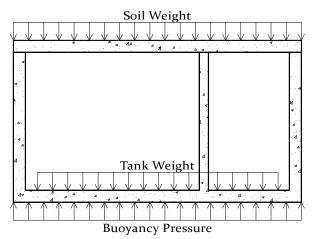
Yes indeed, concrete tanks can f l oat! The following assumptions are made in determining the water level at which f l ot ati on occurs:
