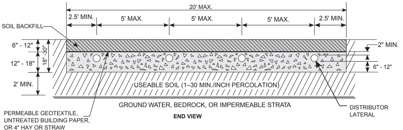
**FIGURE 26: ABSORPTION BED SYSTEM**
