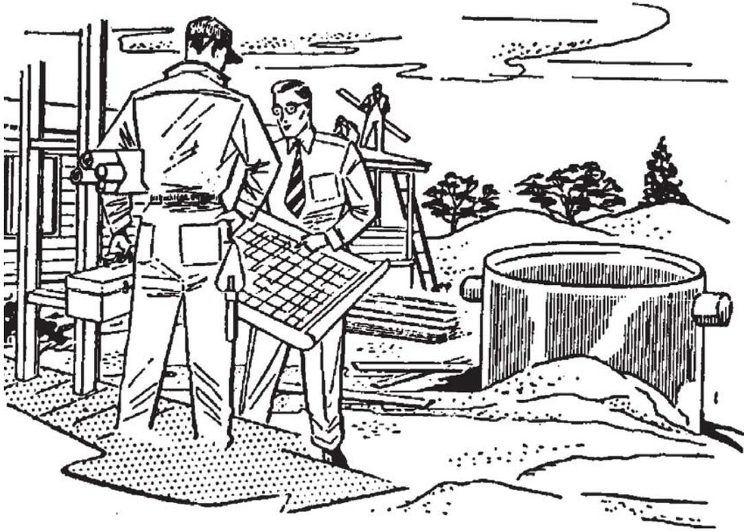
Above all, to properly maintain a disposal field and to assure its longer life, clean the septic tank when necessary. It is better to pump the tank too often than not often enough.
