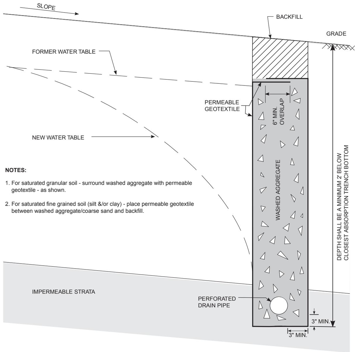
**FIGURE 19: CURTAIN DRAIN - CROSS SECTION**
